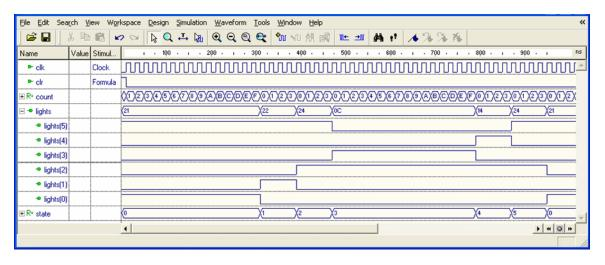
Figure 8.15 Simulation of the VHDL program in Listing 8.4
